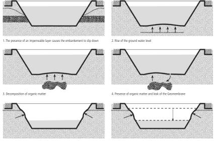
5. Ground water level exceeding the pond water level
